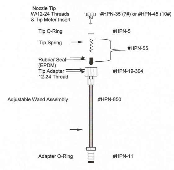
High Pressure Nozzle Assembly Installation
